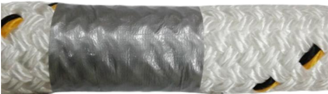
Temporary repair with adhesive tape
