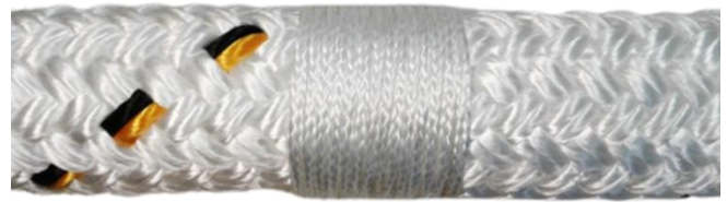
Effective repair by whipping
