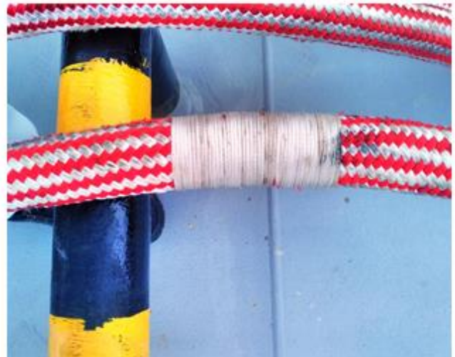
Small repair by whipping
